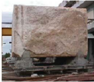
Block before loading into a gang saw
